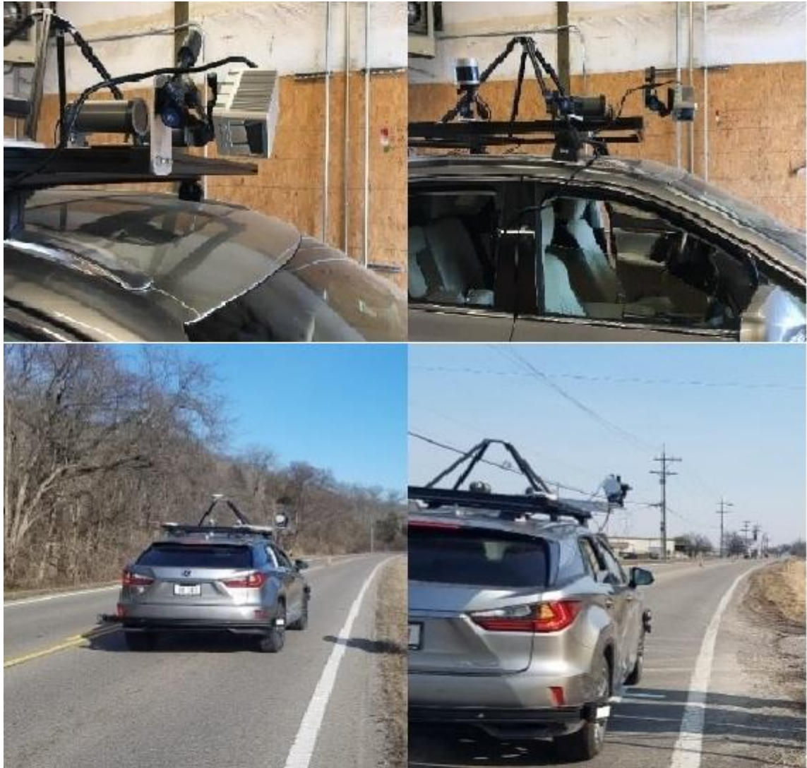
Figure 2: Lidar Sensor and Mounted Camera Setup
