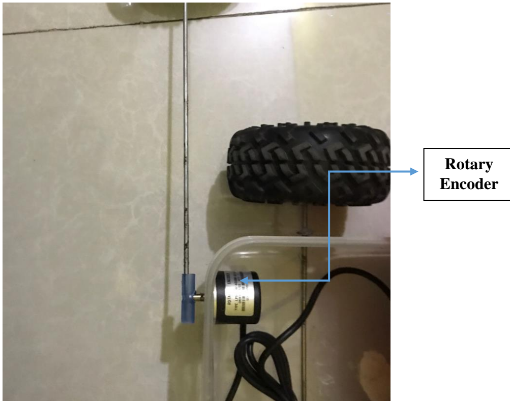
Figure 6: Rotary Encoders for Measuring Height
