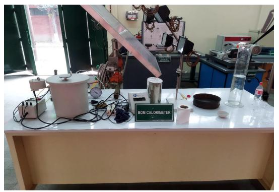
Figure 3. 2: Bomb Calorimeter
