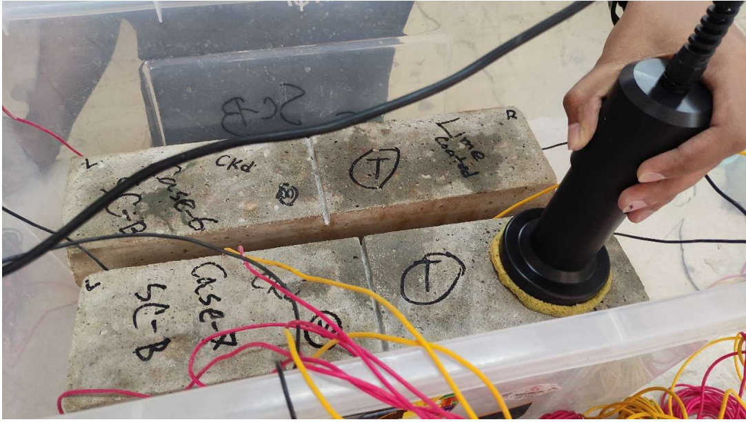
Figure 13: Measurement of micro-cell corrosion
