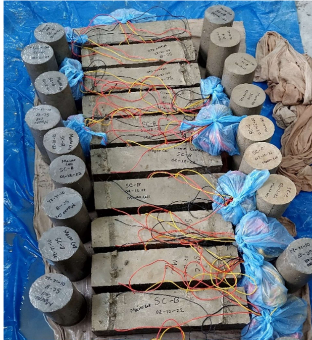
Figure 10: Curing of concrete specimens
