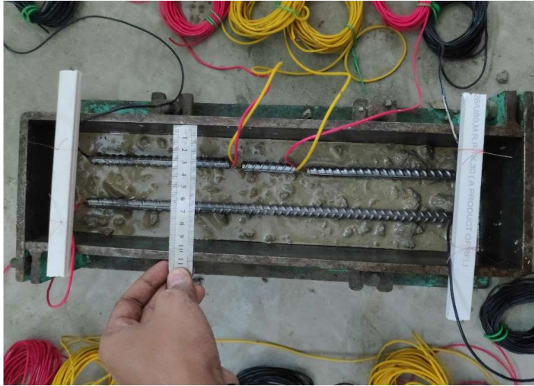
Figure 8: Casting of concrete specimens (placing the rebars)
