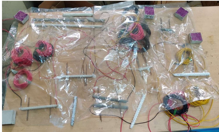
Figure 7: Curing of Coated Steel bars
