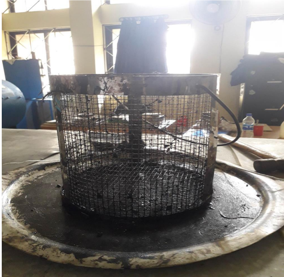
Figure 2: Bitumen Drain down basket
