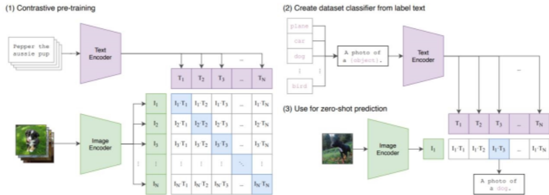
Figure 2.20: The CLIP method, described in the paper by Radford et al. [9], introduces a novel approach for training image and text encoders in a joint manner. Unlike standard image models that focus on predicting specific labels, CLIP trains an image encoder and a text encoder together to predict correct pairings of (image, text) examples in a batch during training. This enables the model to learn a powerful representation of both images and text. During testing, the learned text encoder is used to synthesize a zero-shot linear classifier by embedding the names or descriptions of classes from the target dataset, allowing for accurate classification without the need for fine-tuning. This approach expands the capabilities of the model to understand and relate images and text in a more versatile manner.
