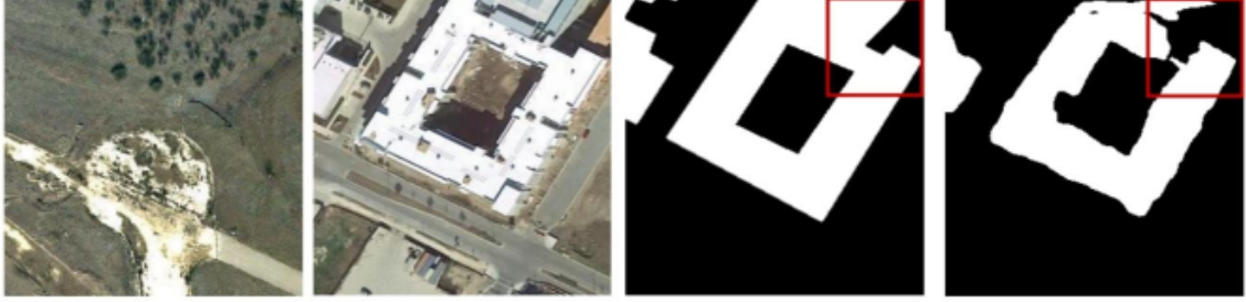
Figure 4.6: Difference between ground truth and predicted images after applying the attention map
