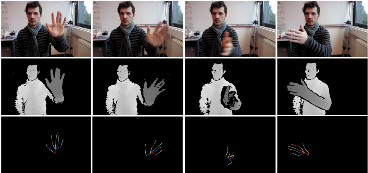
Figure 4.5: Illustration showcasing a swipe left gesture depicted in color (top), depth map representation (middle), and skeletal data visualization (bottom).
