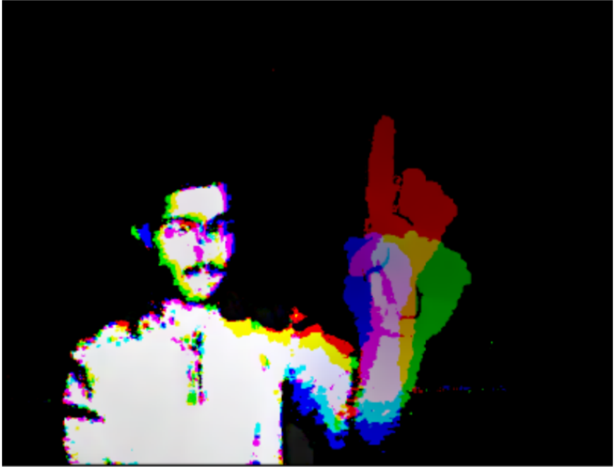
Figure 4.6: Concatenation of three keyframes illustrating a grab gesture.
