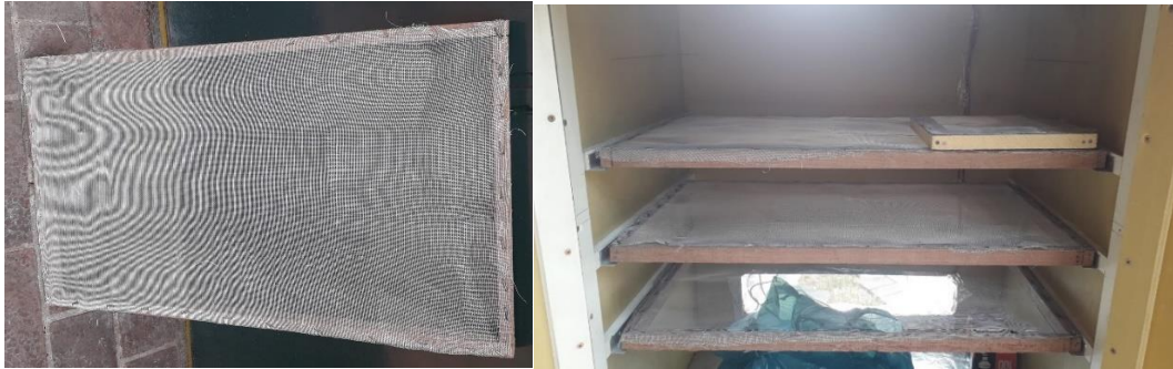
Figure 3.5: Wooden frames and stainless-steel net for trays
