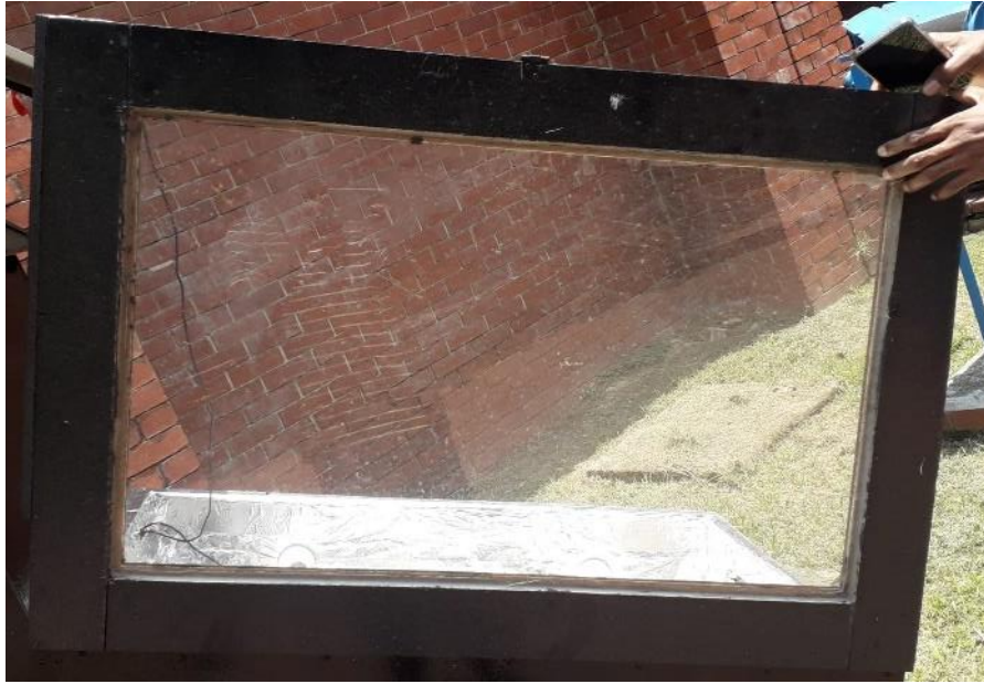
Figure 3.3: Plain Glass for Solar Collector
