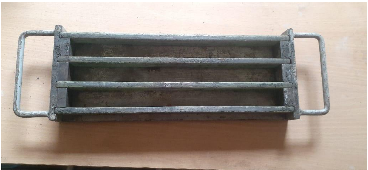
Figure 3.5 Mold for Sorptivity testing specimens
