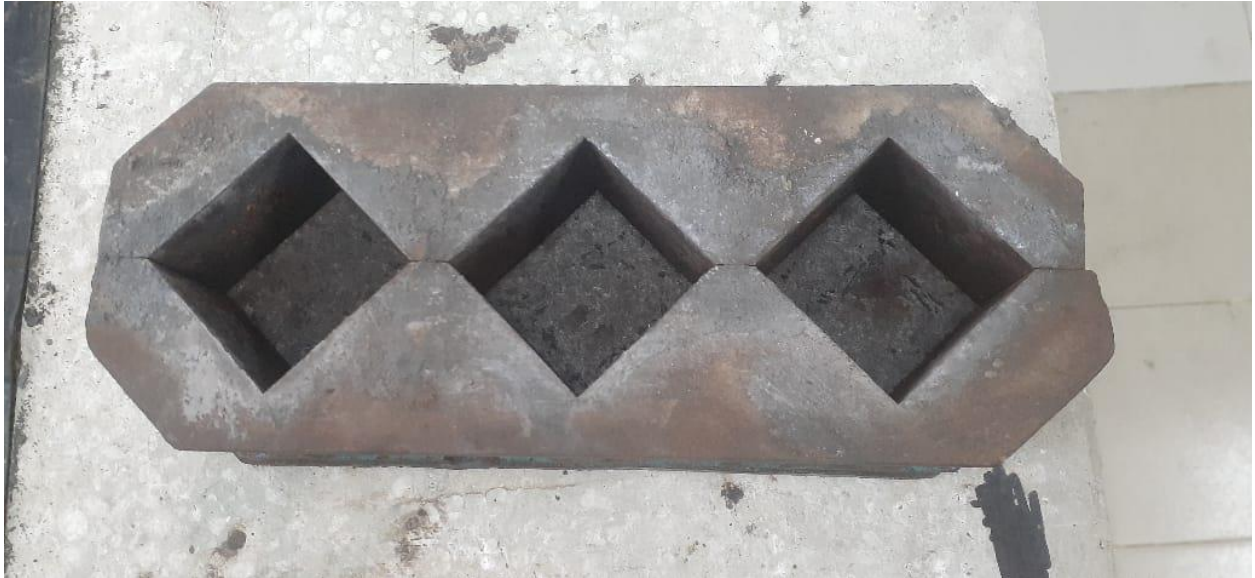
Figure 3.4 Cubic Mold for UHPC Casting
