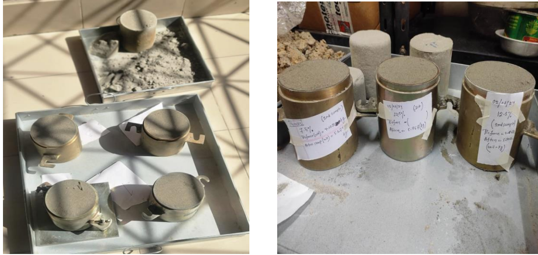
Figure 10 (a): Curing of Blocks before Demolding. (b) Curing of Blocks in Lab condition
