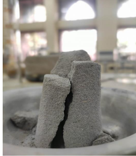
Figure 15(a): Crack gained from UCS Test (b) Brittle condition of 15% Mixture
