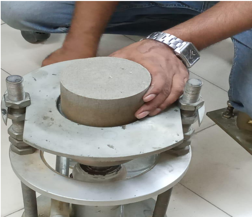
Figure 11: Demolding the blocks with Hydraulic Jack
