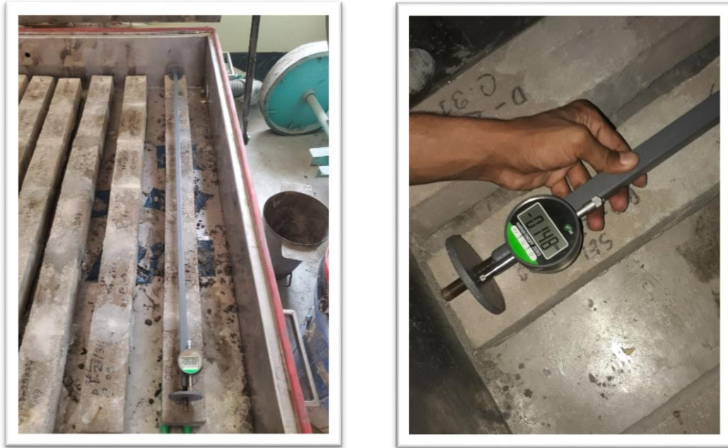
Figure 13: Drying Shrinkage Measurement of Large Sized Specimens
