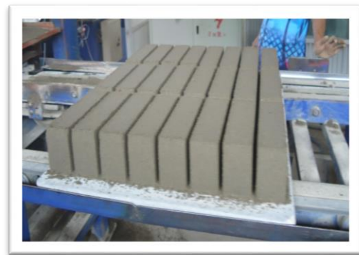
Fresh Concrete Blocks
