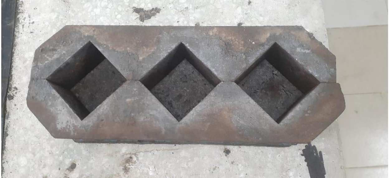
Figure 3.0.4 Cubic Mold for UHPC Casting
