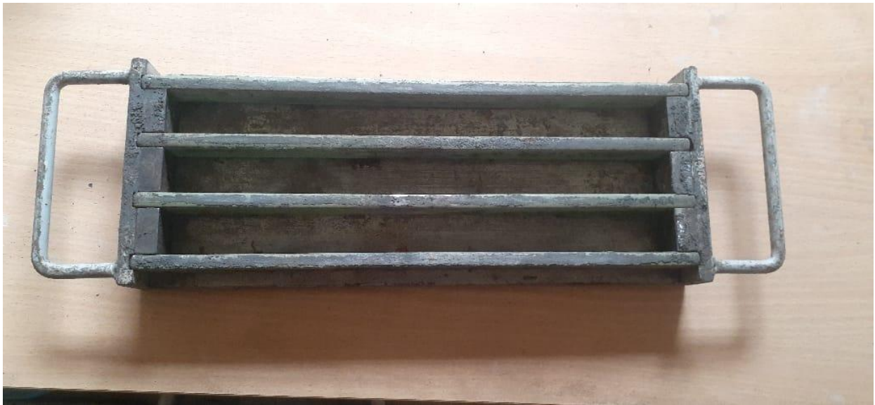
Figure 3.0.5 Mold for Shrinkage testing specimens
