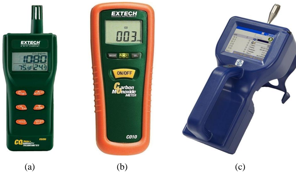
Fig. 3.6: (a) CO 2 meter (Brand EXTECH, USA) (b) CO meter (Brand EXTECH, USA) (c) PM meter (Brand TSI, USA).
