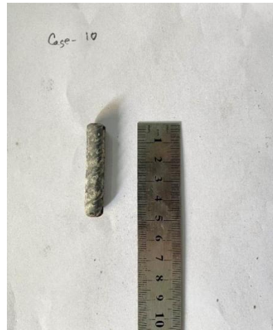
Figure 24: Visual observation of segmented middle steel bar; (a) case 1; (b) case 2; (c) case 9; (d) case 10
