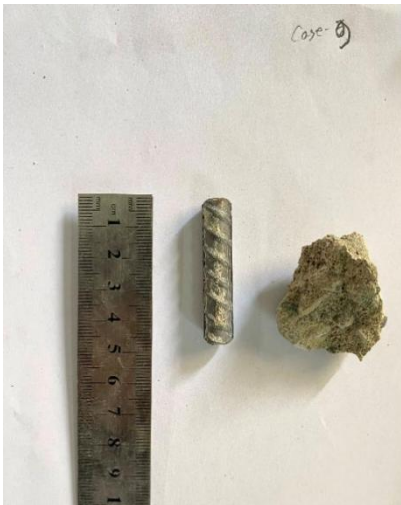
Figure 24: Visual observation of segmented middle steel bar; (a) case 1; (b) case 2; (c) case 9; (d) case 10
