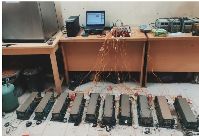
Figure 6: Connection of rebars with data logger
