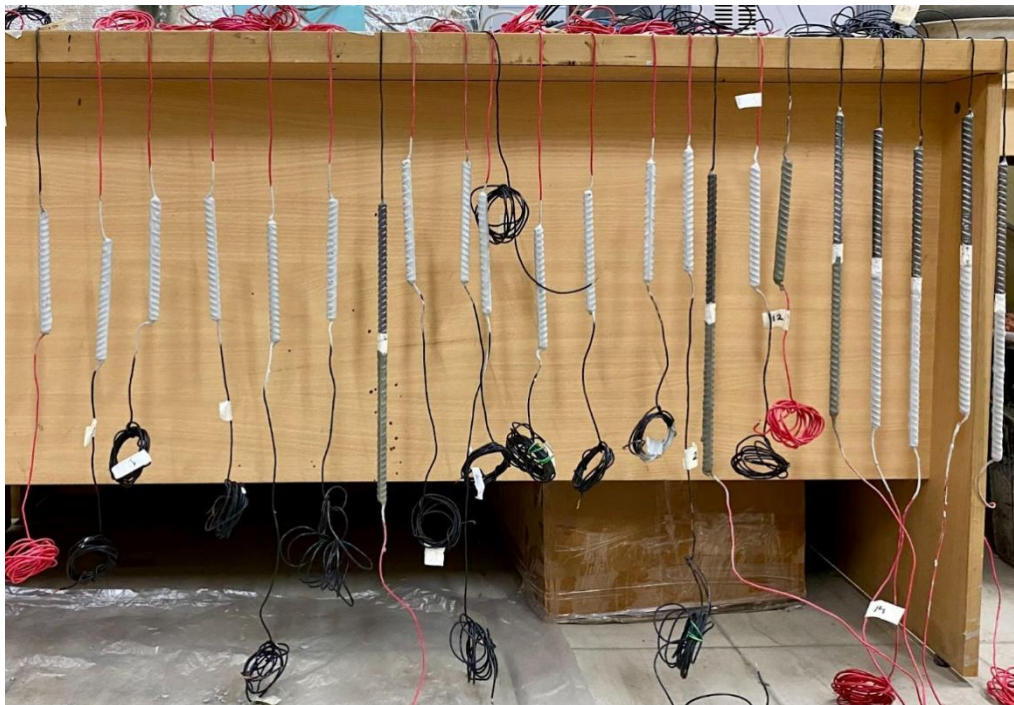
Figure 8: Cement coated rebar and the connection of rebar and wires
