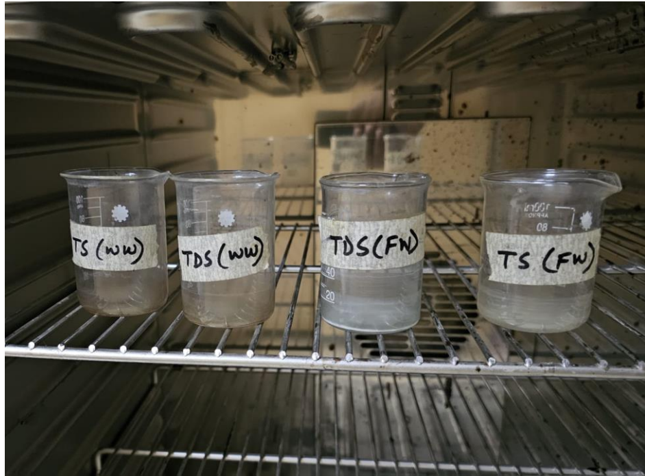
Fig 3.9: Measurement of TS & TDS Manually (Heated at 105 °C for 24 hours)
