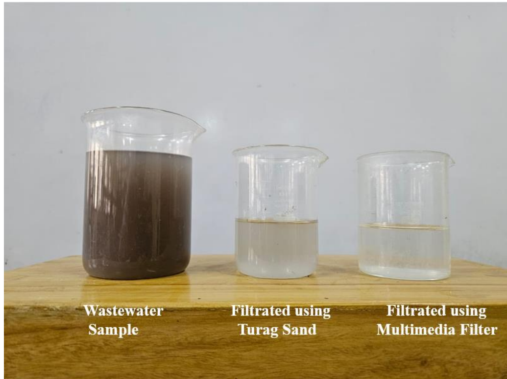
Fig 4.13: Apparent difference between wastewater, Turag Sand filter effluent & Multimedia Filter effluent
