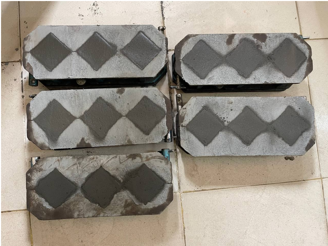
Figure 3.5: Moulding of UHPC mix
