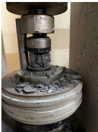
Figure 4.1: Sample Specimen after going through Compression
