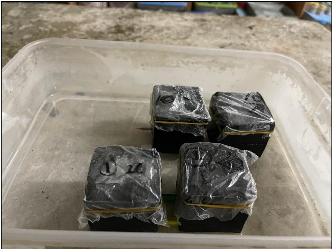
Figure 3.8: Specimen Setup for Sorptivity testing
