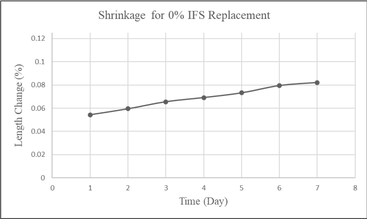
Figure 4.8: Shrinkage Percentage for mix proportion with 0% IFS replacement
