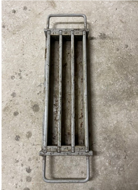
Figure 3.6: Moulding of UHPC mix for Shrinkage
