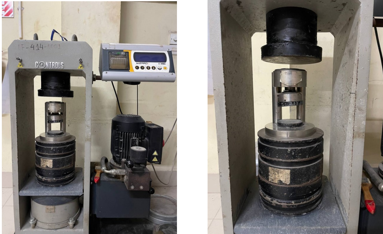
Figure 3.8: Setup for Compressive Strength testing
