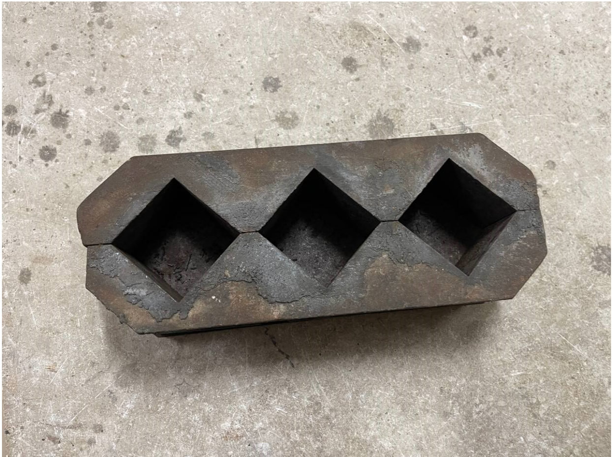
Figure 3.3: Prepared Moulds for UHPC mix
