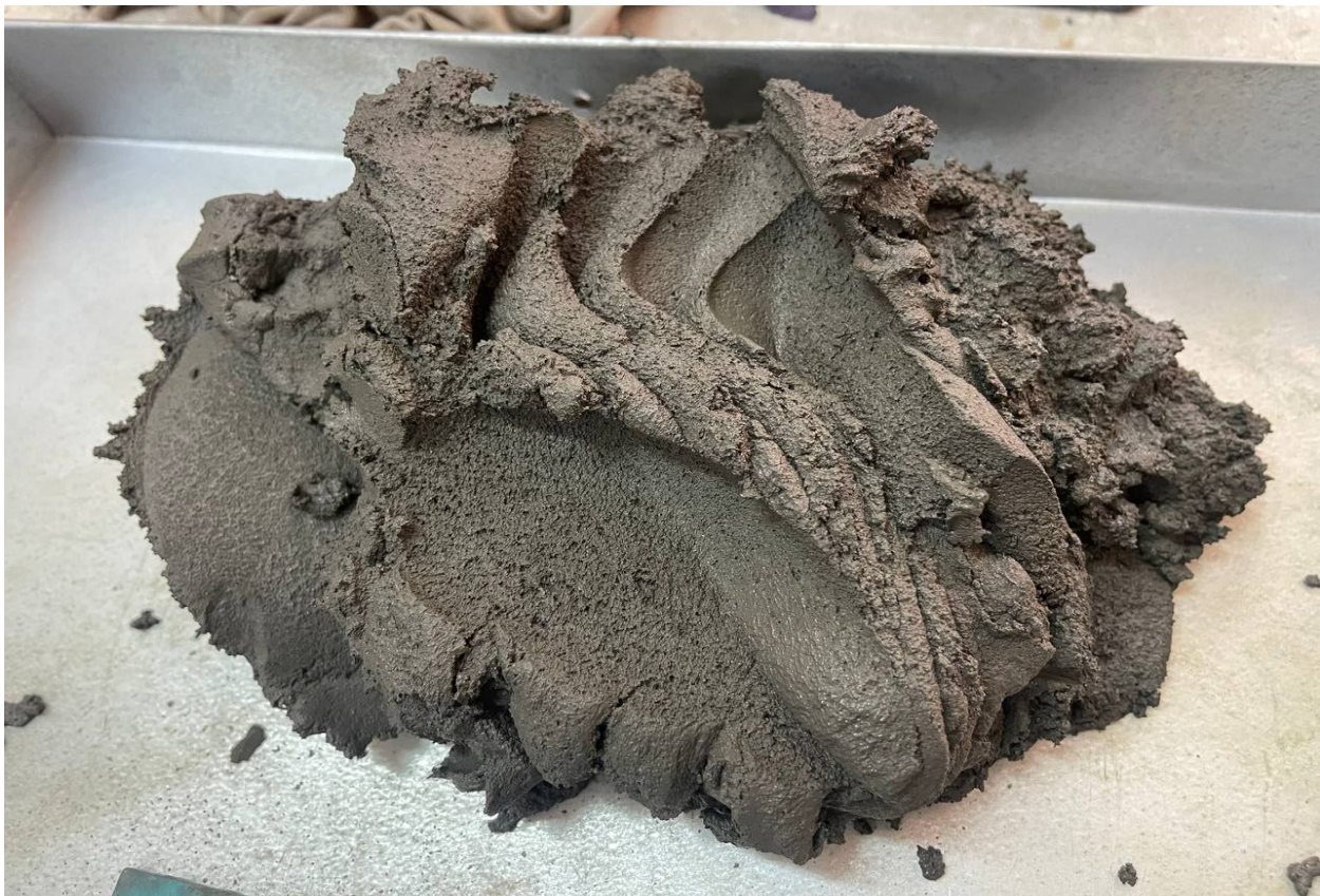
Figure 3.4: Casting of UHPC mix
