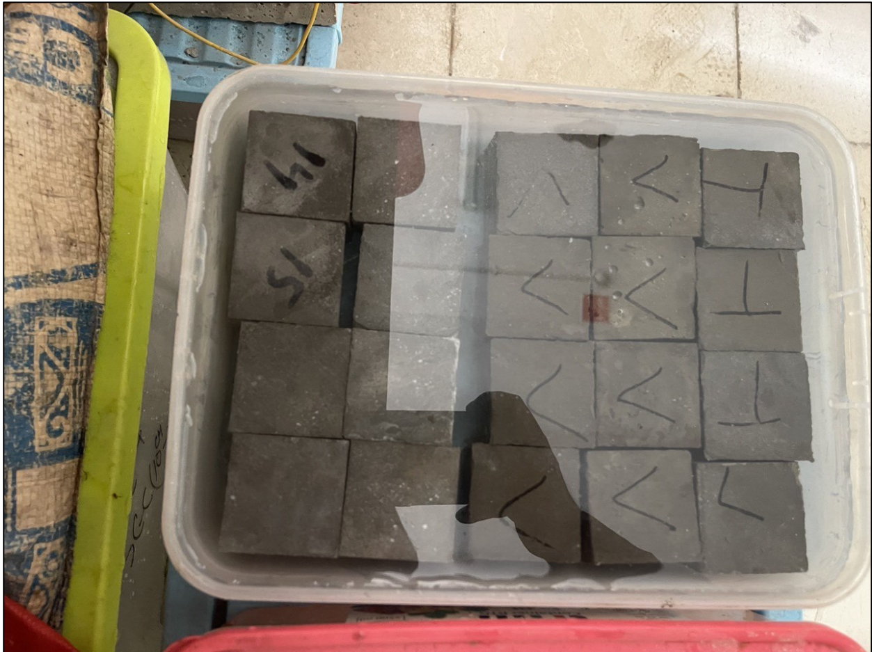
Figure 3.7: Curing of Specimens
