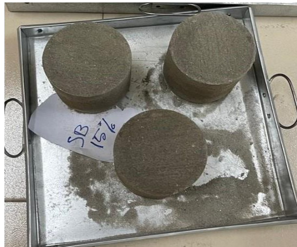
Figure 3-16 UCS samples removing from molds
