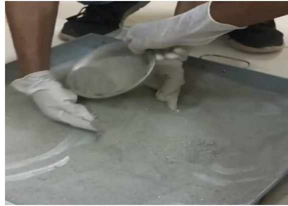
Figure 3-13 Mixing SB-95 with Soil Sample
