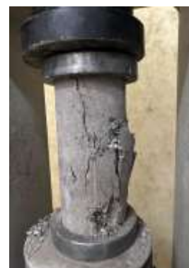
Figure 10: Banana 2 % (Strength 15.89 MPa, 124.85 KN)
