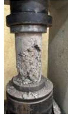
Figure 7: Coconut 1 % (Strength 40.76 MPa, 322.9KN)
