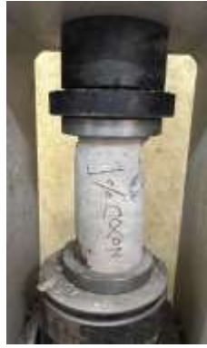
Figure 6: Jute 2% (Strength 16.13 MPa, 270 KN)
