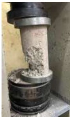
Figure 8: Coconut 2 % (Strength 31.36MPa, 246.6 KN)
