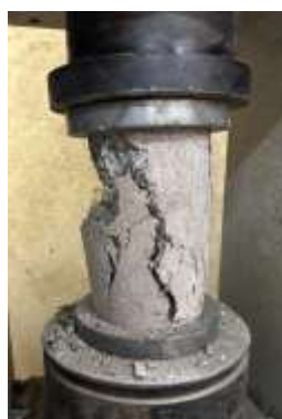
Figure 9: Banana 1 % (Strength 19.11 MPa, 150.5 KN)
