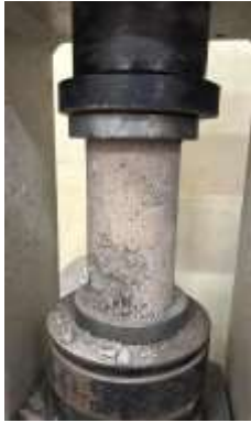
Figure 5: Jute 1 % (Strength 24.2 MPa, 190 KN)
