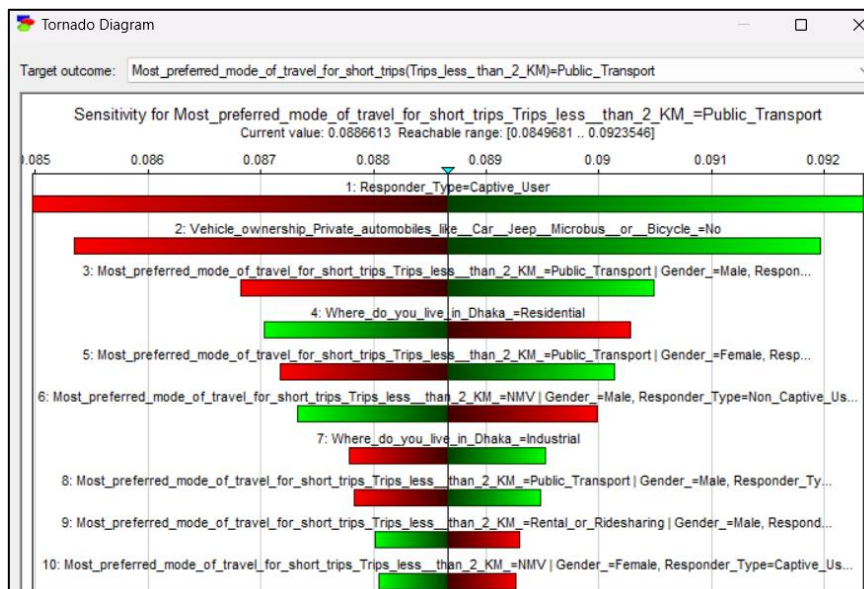
Figure 25: Tornado diagram in sensitivity analysis when the preferred mode is Public Transport for short trip
