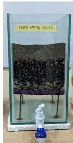
Fig. 3.2: Different layers of multimedia filter
