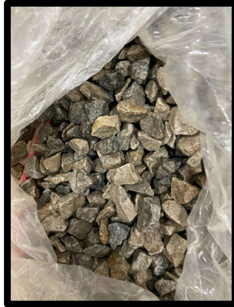
Figure 3.8: Filter media (Coarse Gravel)
