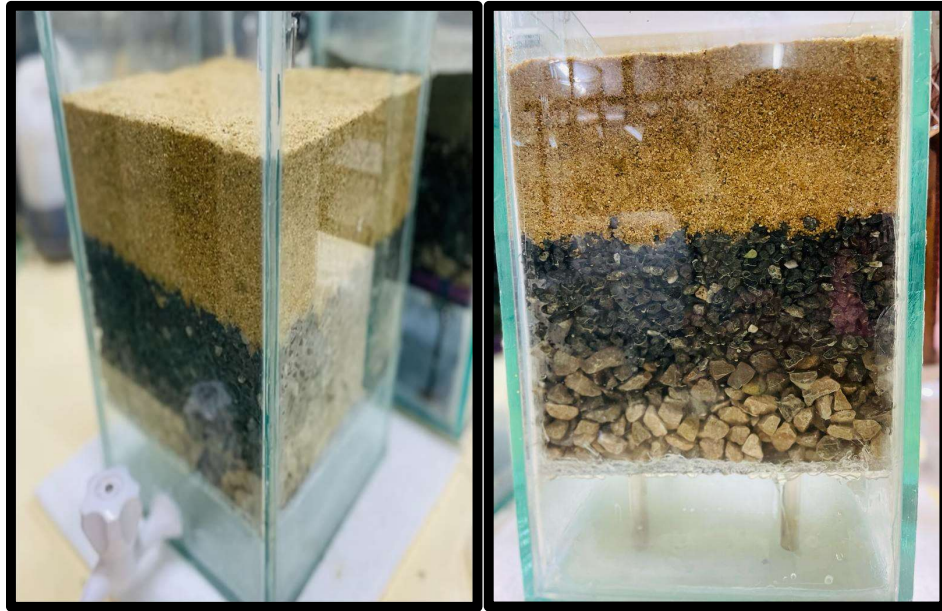
Figure 3.4: Multimedia filter installation and setup
