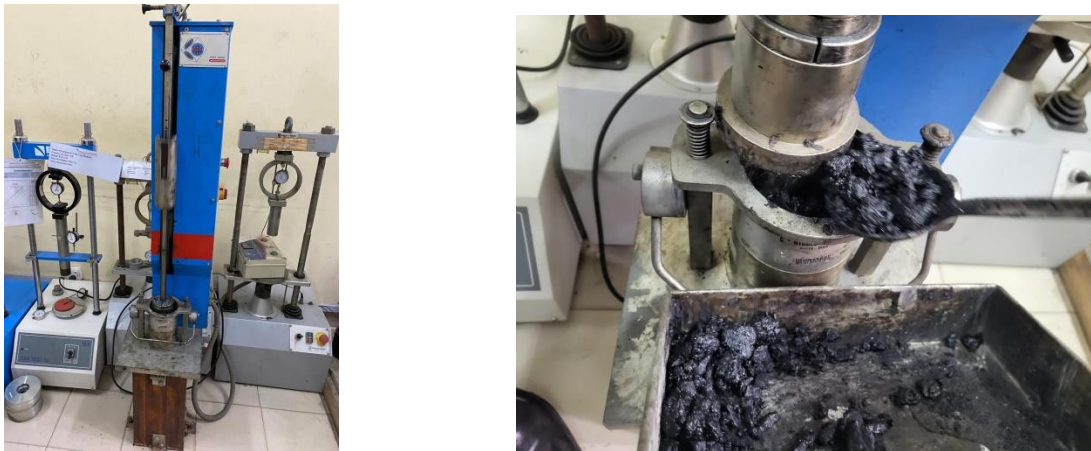
Figure 3: Automatic Compactor and Mold- Collar Adjustment
