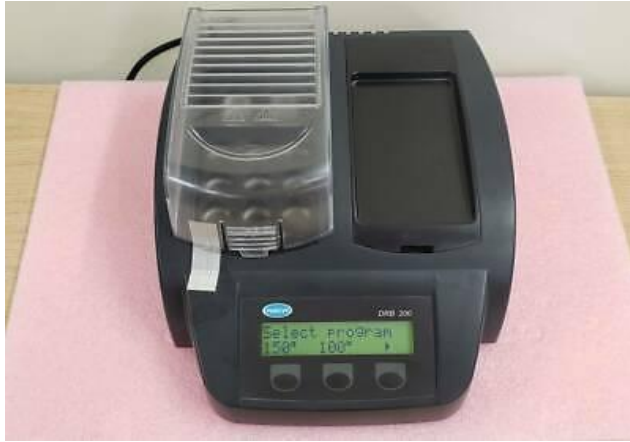
Figure 3.9: COD Reactor Apparatus
