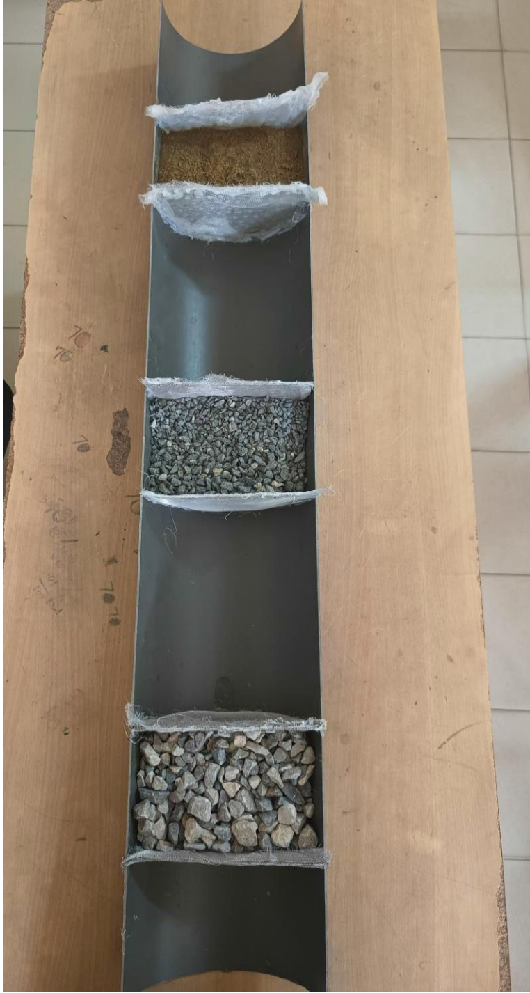
Figure 3.4 : Multimedia Filter ( Top View)
