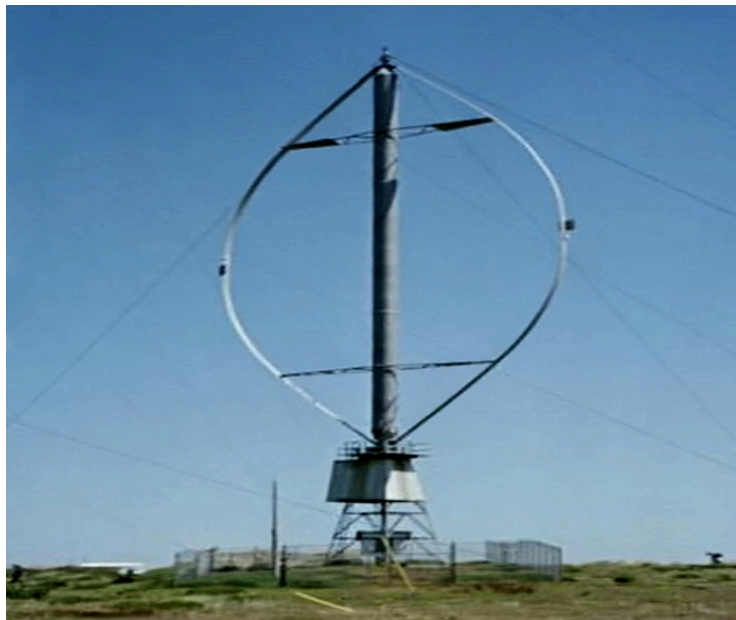
Fig 1.3: Darrieus Wind Turbines[3]
