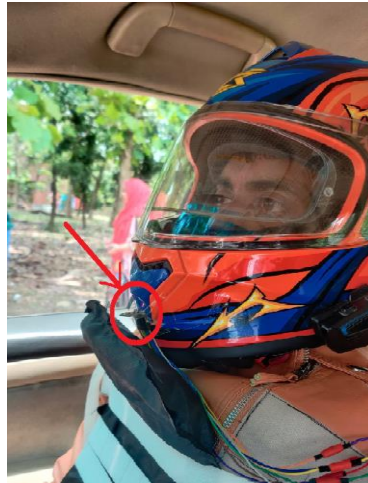
Figure 11: Placement of the sensor on the helmet's periphery while the rider is wearing the modified jacket along with the device
