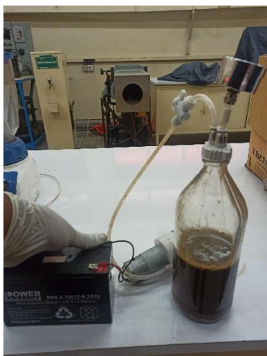
Figure 8: Vacuuming of the digestors and keeping them in black box
