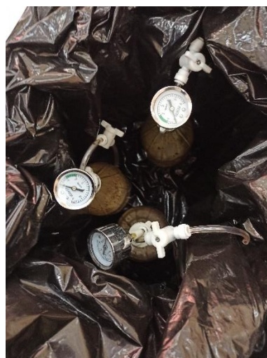
Figure 8: Vacuuming of the digestors and keeping them in black box
