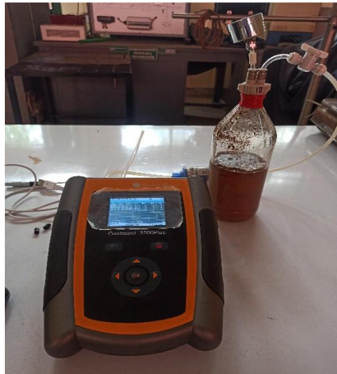
Figure 11: Measuring gas percentage with Gasboard analyzer
