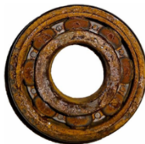
Fig 1.3: Ball Bearing Failure due to Corrosion
