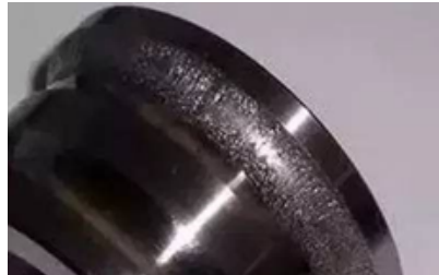
Fig 1.4: Ball Bearing Failure due to fracture
