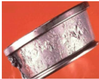
Fig 1.2: Ball Bearing Failure due to fatigue
