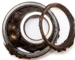
Fig 1.5: Inner race misalignment damage of bearing
