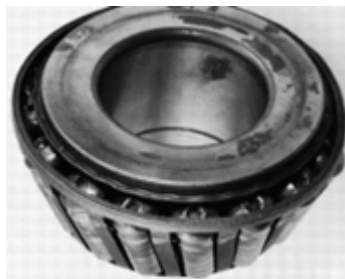
Fig 1.1 Ball Bearing Failure due to wear
