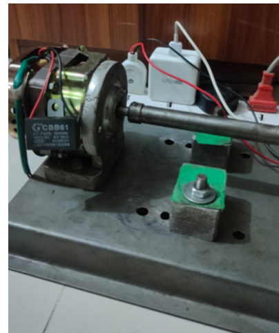
Fig 4.3 Experimental setup running without bearing casing to measure the intensity level of the machine
