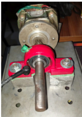
Fig 4.8 Intensity level analysis of new ball bearing
