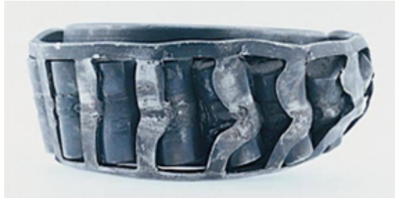
Fig 1.7 Plastic deformation of ball bearing
