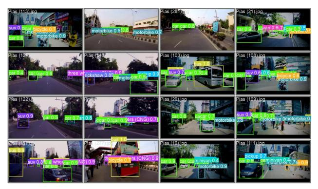
Figure 7 : Prediction Scores Using YOLO v8 medium
