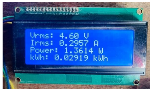
Figure 21 LCD display of Vrms, Irms, Power, kWh
