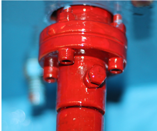
Fig. 3.7: Photograph of the coupling between motor and shaft.
