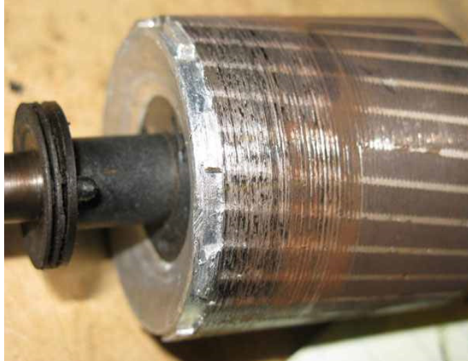
Fig. 2.2: Rubbing of the rotor of a motor.
