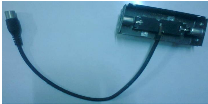
Fig. 3.7: Customized RCA connector we used to connect the probe with the device
