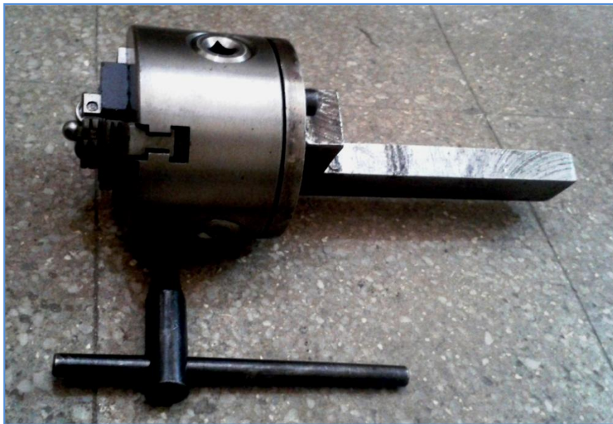
Fig. 4.2 Ball Burnishing Tool
