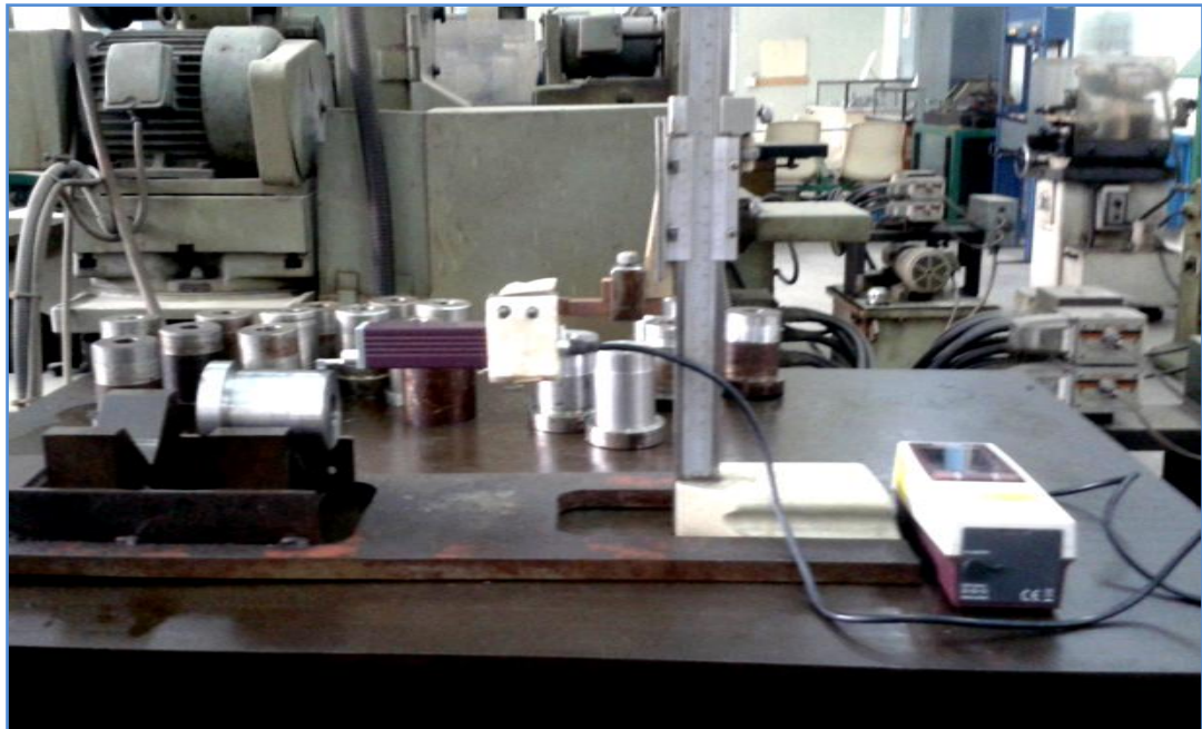
Fig. 4.6 Experimental setup of Surface Roughness measuring device
