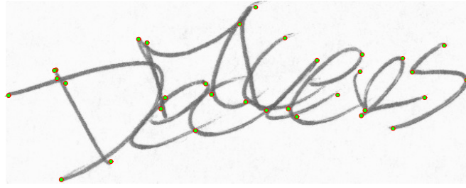
Figure 3.4: Output of Keypoint detection on Chinese Dataset
