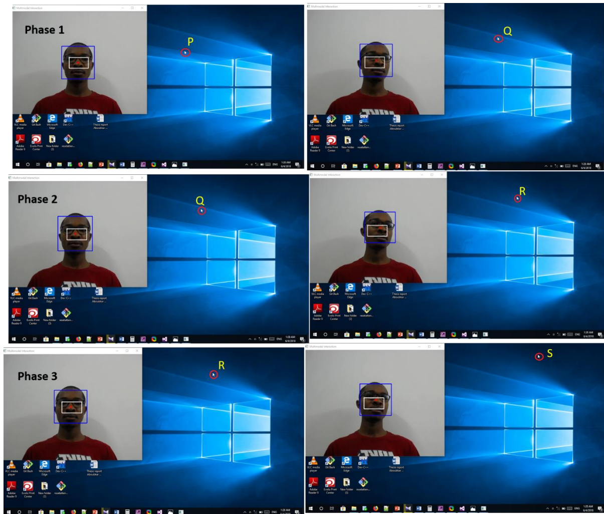
Figure 11: Sequence of break and reset steps to move the mouse pointer from location P to location S
