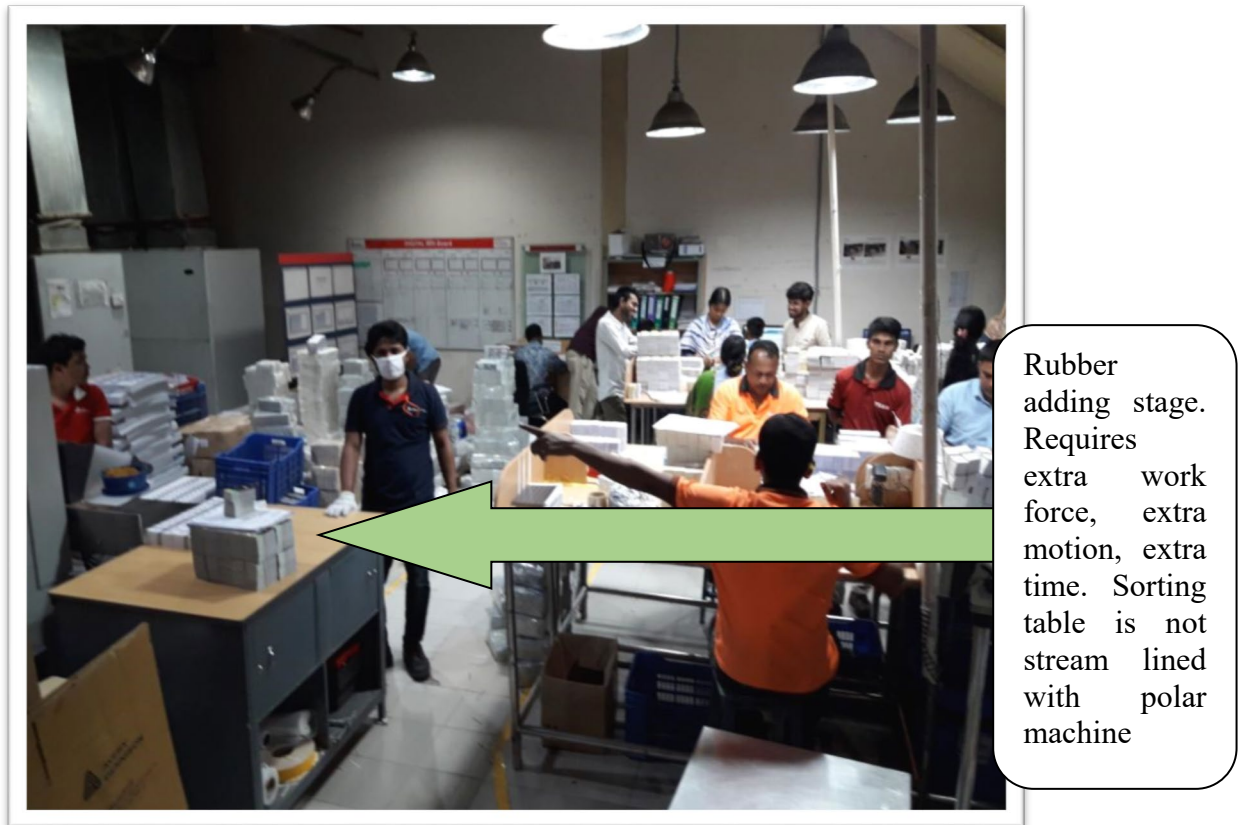
Figure 3.6: Current State Finishing Set up
