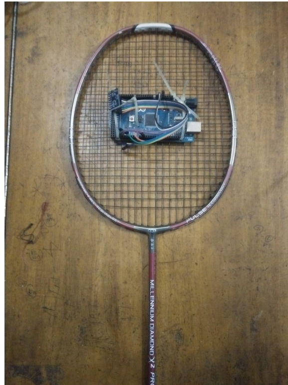
Figure 3.1: Badminton Bat with Integrated Sensor
