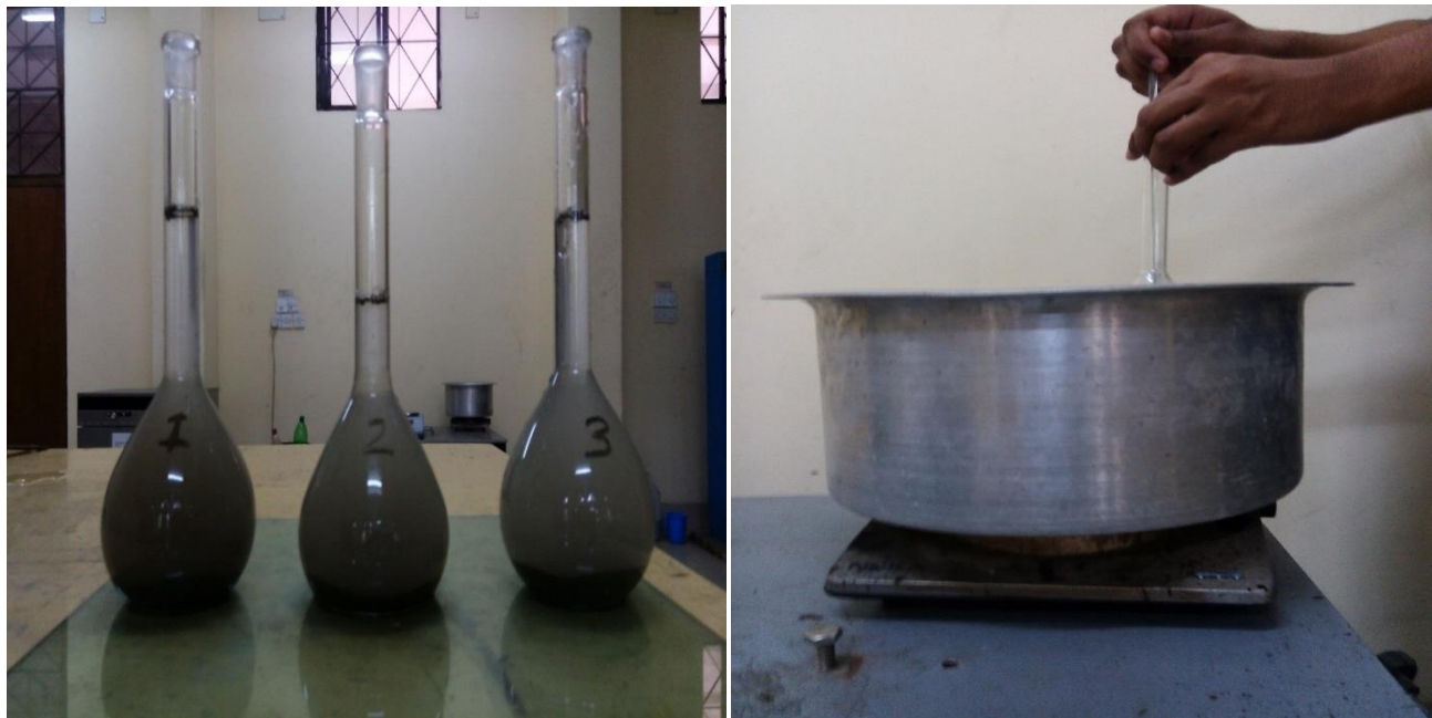
Figure 3.4 Laboratory test of determination of Specific gravity of soil.
