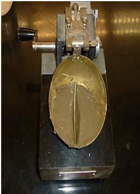
Figure 3.5 Determination of Atterberg Limit of Soil
