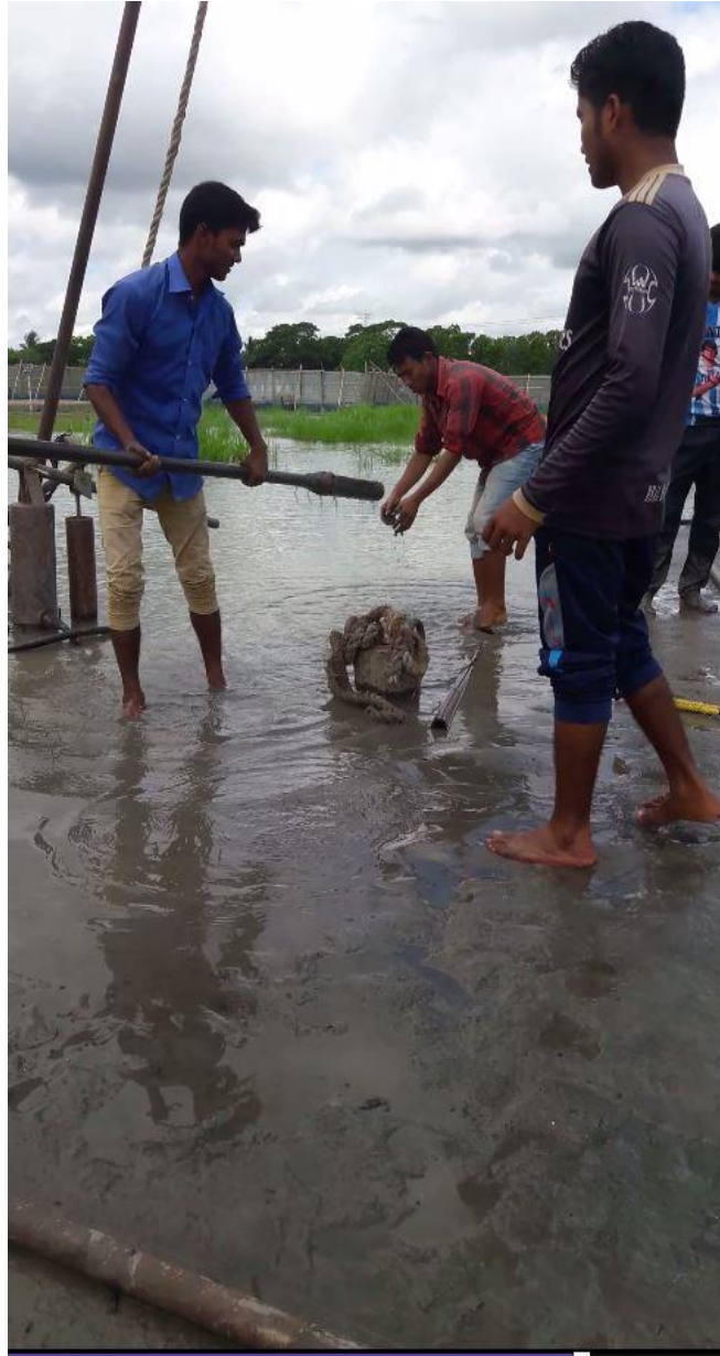
Figure 3.3 Soil sample collection from site and collected undisturbed sample in Shelby tube
