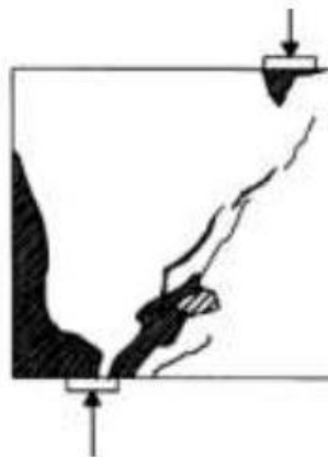
Figure 2.22: Bearing failure (Hong, et al., 2002)
