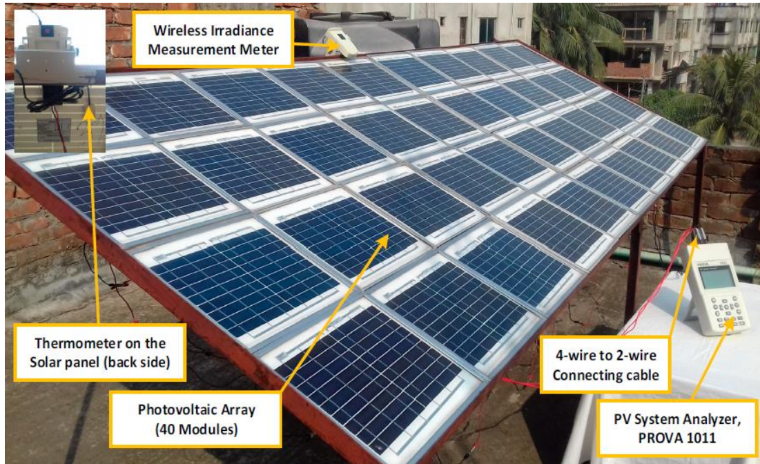
Figure 2.16: Experimental setup of 400 W array at new condition for comparing maximum array output power using different methods of modules arrangement
