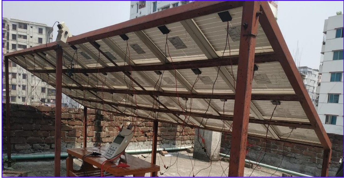
Fig. 3.10: Experimental setup of the non-uniformly aged PV array (back view)
