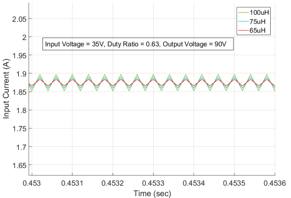
Figure 4.8 Steady state response for three different inductor value when input voltage is 35 V.
