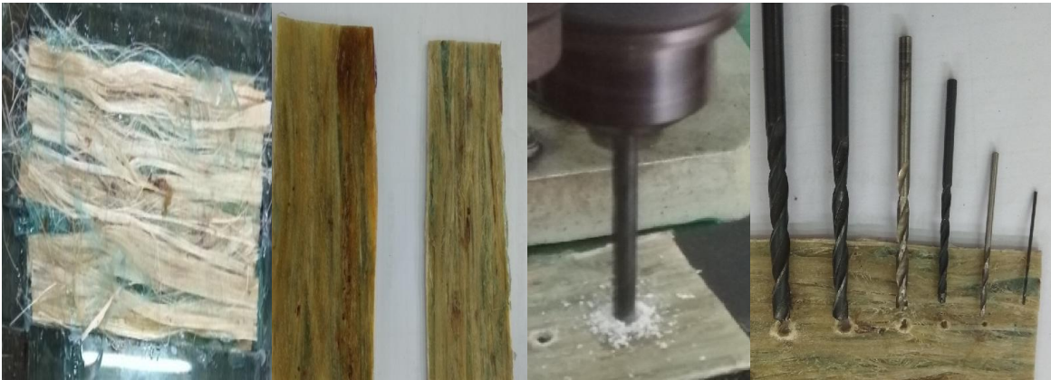
Figure 4.23 Fabrication of natural fiber composite tiles
