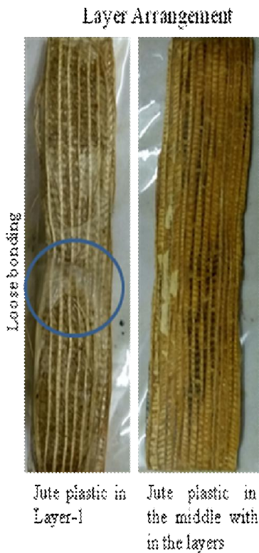
Figure 4.5 Selection of layer arrangement for hand lay and vacuum infusion method
