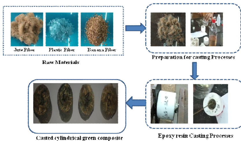
Figure: 3.14 Fabricating steps for casting process
