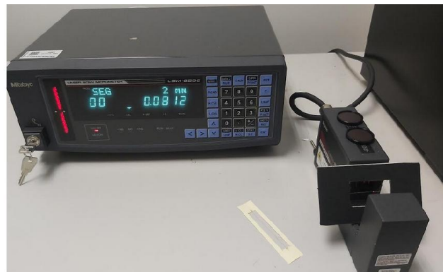
Figure 3.5: Laser Scan Micrometer of Model LSM-500S
