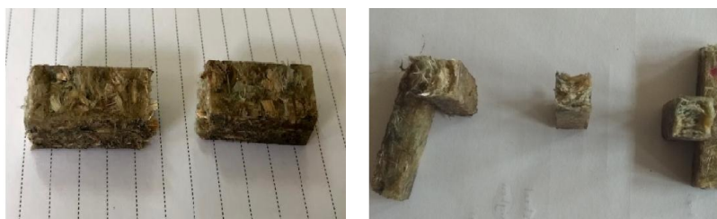
Figure 4.14 Fabricated specimen ruptured behaviour
