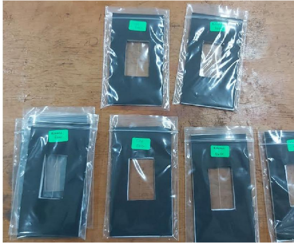
Figure 3.7 Fiber gripper with multi-layer hard board.
