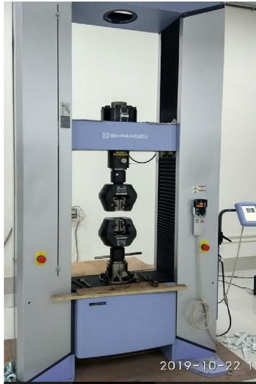
Figure 3.8 Universal testing instruments, model AG-X plus series
