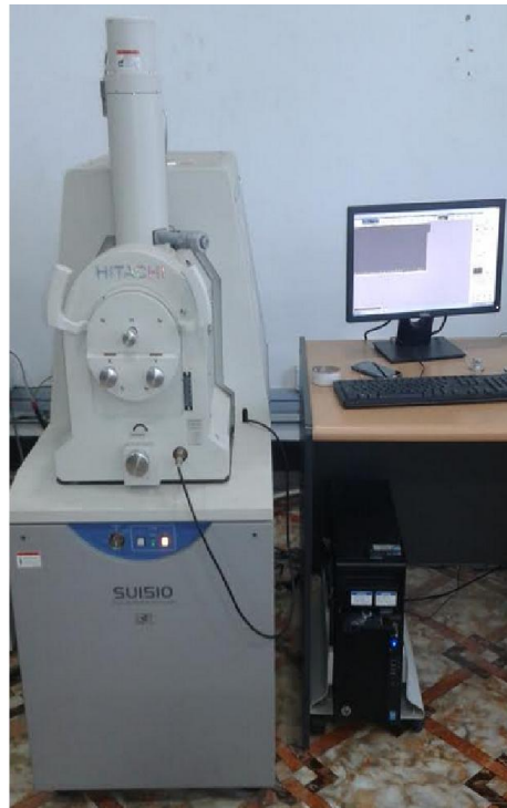
Figure 3.2 Scanning Electron Microscope of SUI510 model
