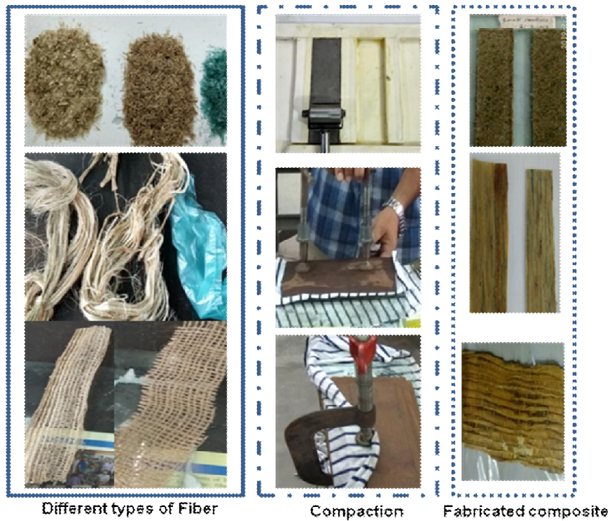
Figure 3.13: Process sequence of hand lay method for different composite
