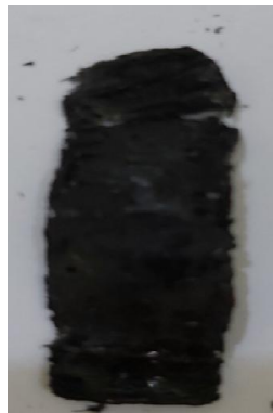
Figure 4.27: Burnt composite of charred black.
