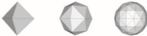
Figure 1. Decomposition of the Earth's surface for triangular meshes with resolutions of zero, one, and two.
