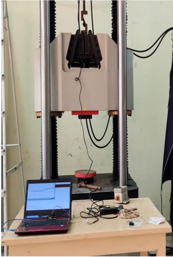
Figures: Tensile and Shear stress is applying in our sample through UTM.
