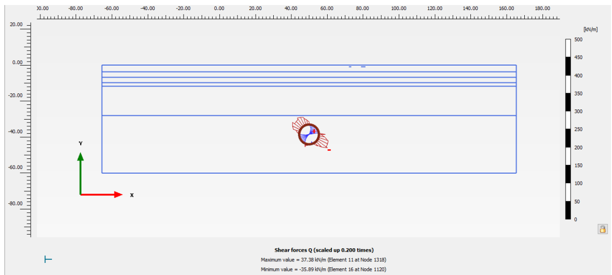
Figure 5.3.2.3: Shear force diagram of tunnel (CASE 2 – Tunnel under center of the road)
