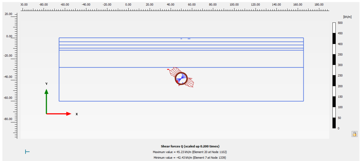
Figure 5.3.2.2: Shear force diagram of tunnel (CASE 1)
