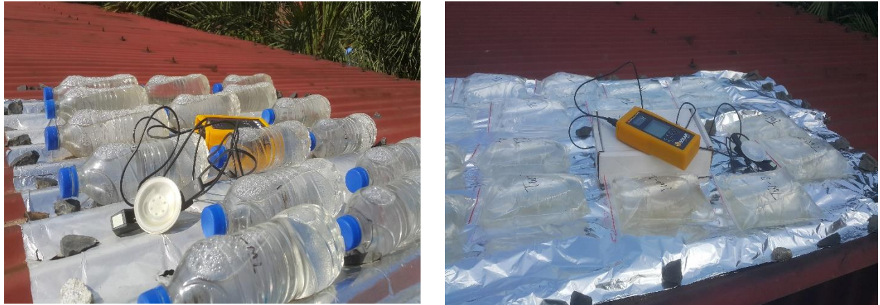
Figure 3. 5. Diagram showing the test water samples to direct sunlight at rooftop in SODIS system.
