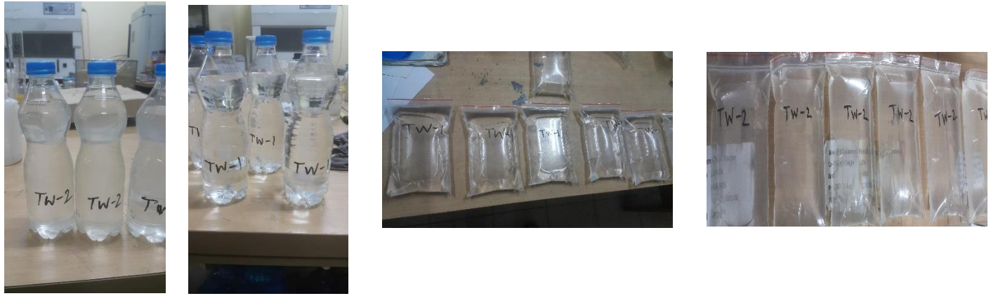
Figure 3. 4. Test water-1 and Test water-2 prepared in PET bottle and plastic bag.
