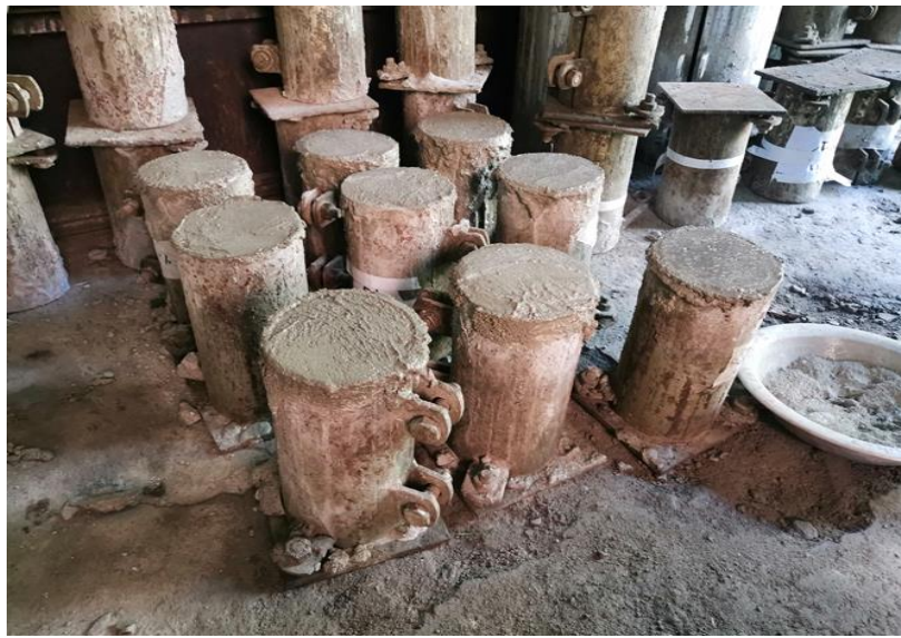
Figure : Cylinders after casting
