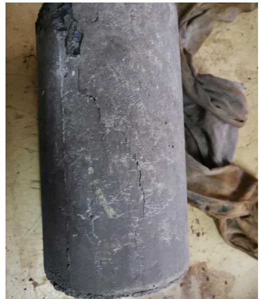
Figure : 0% RAP used (Virgin Material) cylinder compressive strength cracking
