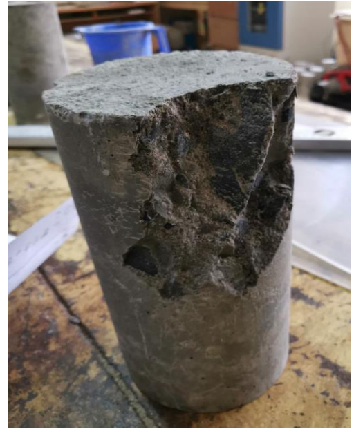
Figure : 60% RAP used cylinder compressive strength cracking
