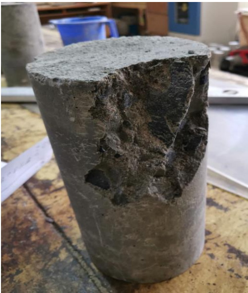
Figure : 30 % RAP used cylinder compressive strength cracking
