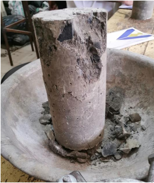
Figure : 100 % RAP used cylinder compressive strength cracking
