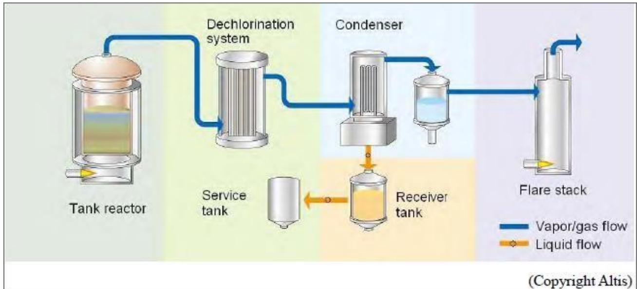
Figure : Schematic diagram of a plant for medical wastes
