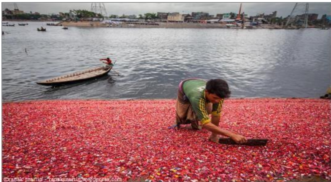
Figure: Drying the flakes (Martin, R (2014). Plastic recycling workers in Bangladesh, Ranak Martin blog, 17.11.2014)
