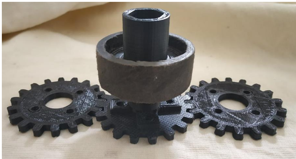
Figure 4-5: Custom made 3D printed gear
