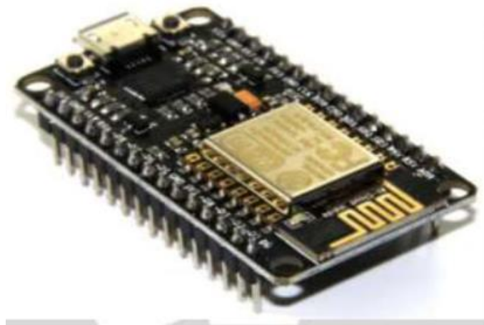
Figure 2: ESP8266 WIFI MODULE
