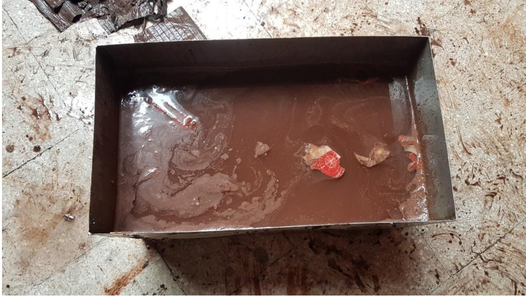
Figure 07: Hydro-separator filled with water and plastic bits floating up
