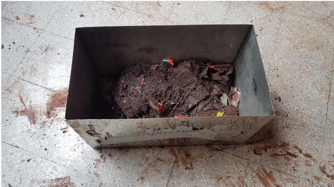
Figure 06: Crushed battery bits inside the hydro-separator
