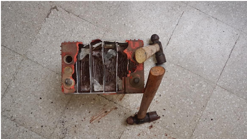
Figure 05: The battery being crushed using hammers
